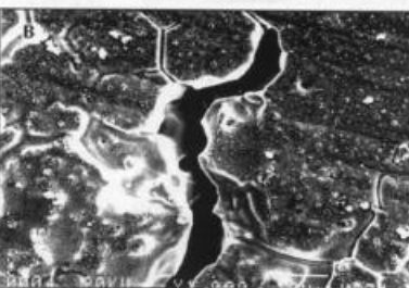
Fig. 15 — Morphology of HAZ cracking in as-tested condition. A — Heat 1356; B — Heat 1358.
