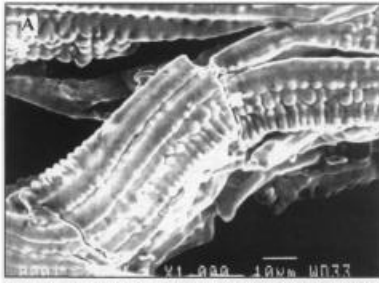
Fig. 10 — SEM images of typical fusion zone crack morphology in as-tested condition. A — Heat 1356; B — Heat 1358. 3000X.
